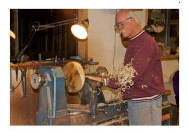
He then began creating a bowl shape on the lathe. Jerry has a video camera and monitor set up so everyone got a clear view of his work. He showed the use of the various gouges used to shape the wood: a bowl gouge - a deep fluted gouge used to turn the outside and inside of bowls and vessels. Often these gouges have a thick shaft and long handle. There is also the spindle gouge or detail gouge - a shallow fluted gouge used to create details on spindles,
